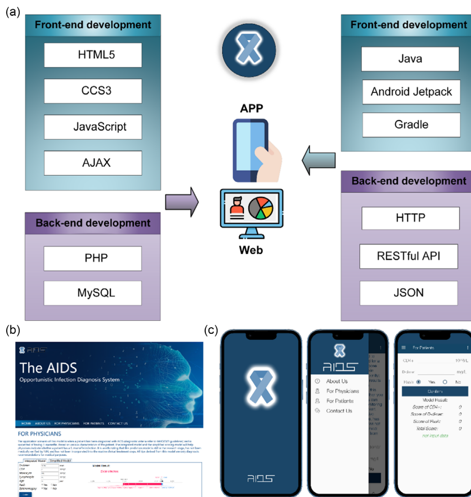
Figure 7. Web and app development result diagram. a) The workflow of creating the web and app page. b) Display of our free web platform. Building upon our preliminary infection screening model, we have devised a complimentary web-based platform to facilitate early detection of Talaromyces marneffei infection among medical professionals and patients alike. c) Display of our free app platform. To overcome constraints related to time, location, and equipment, our team has developed a versatile mobile application. This application is specifically designed for seamless integration and use within the Android operating system.
